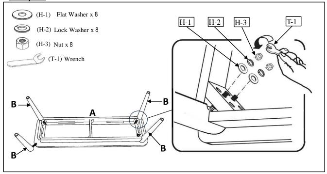
Place the Bench Top (A) upside down onto a padded, non-marring surface. Position the Legs (B) at each corner of the Bench Top (A) by inserting the hanger bolts through the holes. Secure by engaging Flat Washers (H-1), Lock Washers (H-2) and Nuts (H-3), stacking the hardware in the order as shown. Once engaged, fully tighten using the provided Wrench (T-1). DO NOT OVERTIGHTEN. Repeat for all Legs (B).
